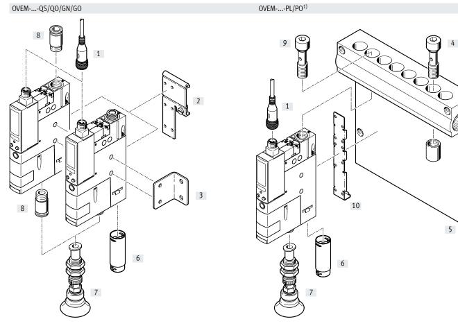
1) Hollow bolt [9] and mounting bracket [10] are included in the scope of delivery for the OVEM-...-PL/PO.
