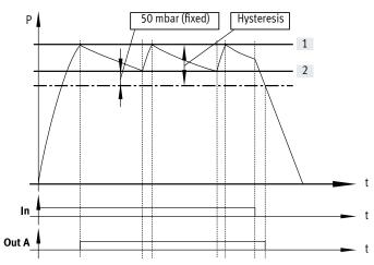
Air saving function (with OVEM-...-OE/OPE/CE/CPE-...-1PD/2P/2N/PU/PI/LK)
