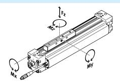
If the drive is subjected to two or more of the indicated forces and torques simultaneously, the following equation must be satisfied in addition to the indicated maximum loads:
