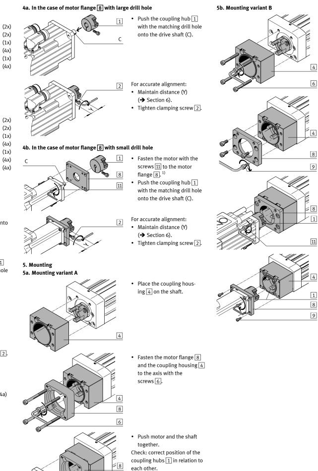
Fasten the motor with the screws 11 to the motor
