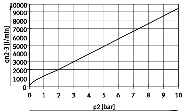
Flow rate q_n from 2 \rightarrow 3 as a function of output pressure p_2
